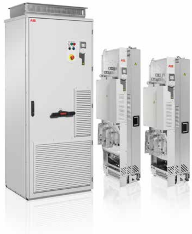
ACS580-04 drive modules with IP00 protection class extend the power range from 250 to 500 kW, and voltage range from 380 to 480 V. The modules are available in frame sizes R10 and R11. The cabinet-built drives have the IP42 protection class as standard.
