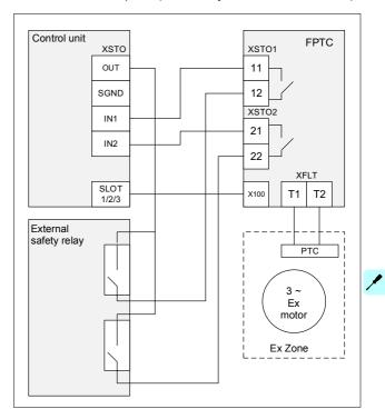
One-channel connection. This connection is SIL1 capable (no redundancy between STO channels).
