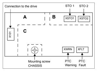
There is reinforced insulation between isolation areas A and C as well as between isolation areas B and C.
