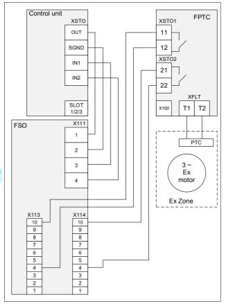
With an external safety relay, two-channel connection. This connection is SIL2 capable (redundancy between STO channels).
