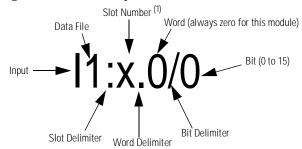
(1) I/O located on the controller (embedded I/O) is slot 0. I/O added to the controller (expansion I/O) begins with slot 1.
