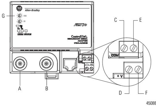
1. Connect the ControlNet network cable to connector, terminal A.
