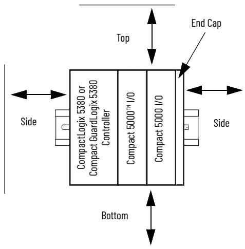
**IMPORTANT** If Compact 5000 I/O modules are installed next to a CompactLogix 5380 or Compact GuardLogix 5380, or CompactLogix 5480 controller, you must mount the system horizontally.
