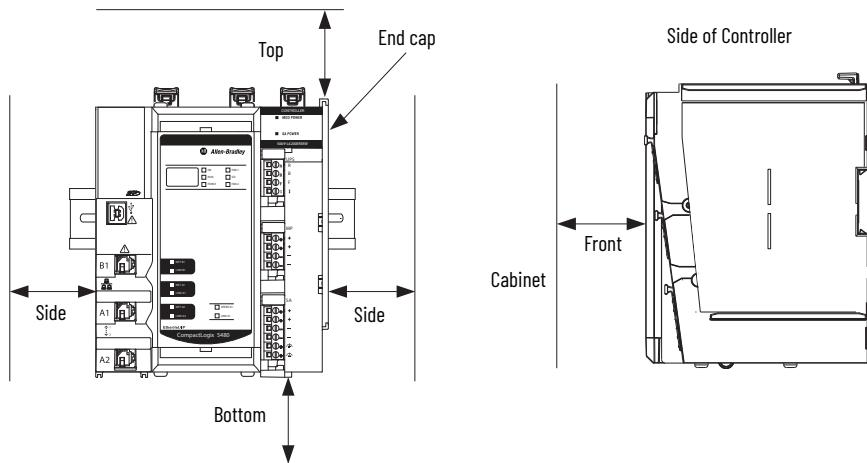
**IMPORTANT** If Compact 5000 I/O modules are installed next to a CompactLogix 5380, Compact GuardLogix 5380, or CompactLogix 5480 controller, you must mount the system horizontally.
