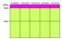
In this operating mode the capacity of the DC link of the brake module is reduced by approx. 10%. At 90% DC link load the brake chopper then directs the generated braking energy to the external brake resistor and, when this has reached its capacity limit, into the internal brake resistor.
