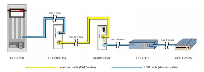
The third configuration (3) has nearly the same structure than configuration 2. The USB hub is connected after the extension. The maximal distance is also 61 meters: 1 meter of cable from USB host to the USB extension box CU8800; up to 50 meters extension cable; 5 meters from extension box to USB hub and 5 meters of cable to the USB device.
