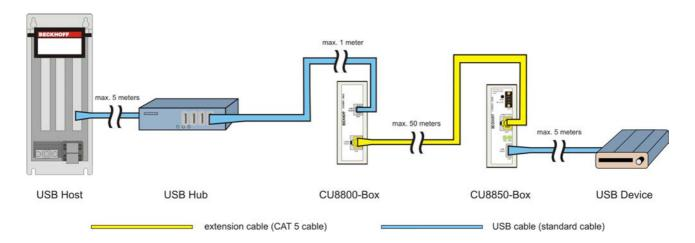
This configuration (2) contains an additional USB hub. The USB hub is connected directly to the host computer. The maximal distance of extension is 61 meters: 5 meters of cable from USB host to the USB hub; 1 meter cable to the extension box CU8800; up to 50 meters extension cable and 5 meters from extension box to USB device.
