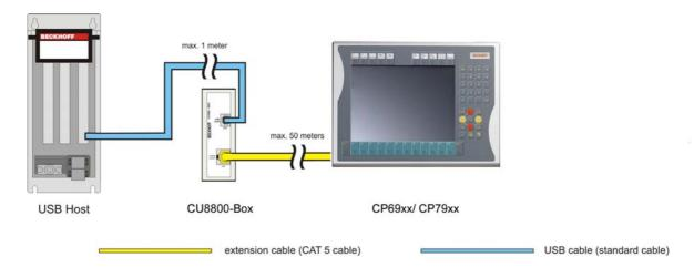
This configuration shows a CP69xx/ CP79xx Control Panel connected to the CU8800 extension box. The maximal distance of extension is 51 meters: 1 meter of cable from the host computer to the CU8800 extension box; up to 50 meters extension cable to the Control Panel.
