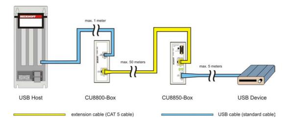
This configuration (1) contains no additional USB hub. The maximal distance of extension is 56 meters: 1 meter of cable to the extension box CU8800; up to 50 meters extension cable and 5 meters from extension box to USB device.
