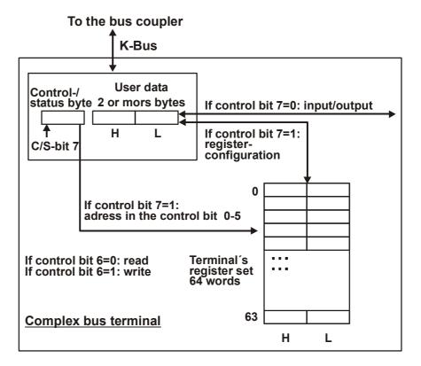
The control or status byte occupies the lowest address of a logical channel. The corresponding register values are located in the following 2 data bytes. (The BK2000 is an exception: here, an unused data byte is inserted after the control or status byte, and the register value is therefore placed on a word boundary). Example 1
