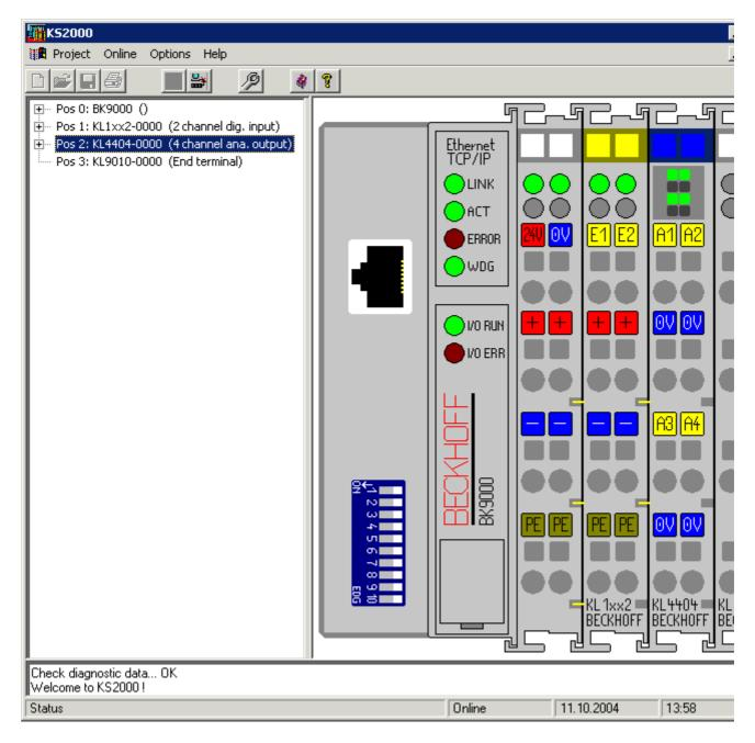
The left-hand KS2000 window displays the terminals of the fieldbus station in a tree structure. The right-hand KS2000 window contains a graphic display of the fieldbus station terminals.
