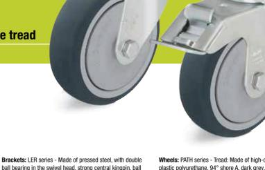
Brackets: LER series - Made of pressed steel, with double ball bearing in the swivel head, strong central kingpin, ball protection by the special top plate and ball disc design. The special Blickle dynamic riveting process of the swivel head results in minimal swivel head play and smooth rolling characteristics with an increased service life achieved by the work hardening of the ball race grooves. Rolted wheel axle
