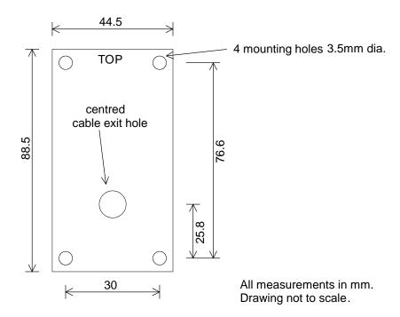
If the spacer plate is used the reader cable may be brought out of one of four exit points on the spacer: top, bottom, left or right. This enables the cable to be run on the surface of the wall. If no spacer plate is used a minimum hole size of 6.5mm must be drilled in the wall at the cable exit position as shown above to allow the cable to exit perpendicular to the reader.
