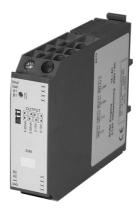
The current measurand transducer BIM serves the capture and dc isolation of an alternating current and following transformation in an impressed current or tension signal. The measurand transducer has a three way isolation, i.e. dc isolation between input/output and supply tension. The choice of the output signals (0-10 VDC, 2-10 VDC, 0-20 mA or 4-20 mA) is made about a frontal 2-pole DIP switch. A green LED shows the ready status.
