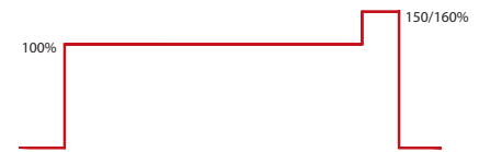
Typical braking profile for vertical motion (40% duty cycle)
