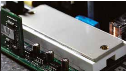
Integrated heat control in IGBT
