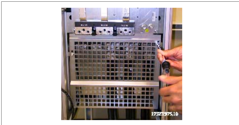
Illustration 3.81: Mounting of EMC shield.
