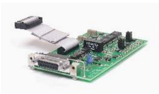
An ISO AMP CARD should be used in case of a non-floating programming source.
