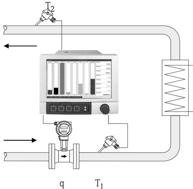
$$E = q \cdot \rho(T_1) \cdot [h(T_1) - h(T_2)]$$
