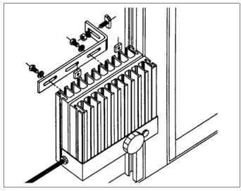
The mounting bracket and all shown bolts and nuts are supplied with the heater.
