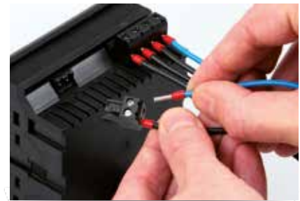
Fig.: Pluggable screw terminals for easy connection
