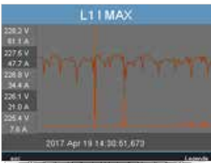
Fig.: Illustration of the full wave effective values for an event (voltage drop)
