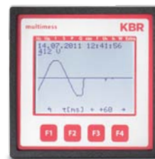
Graphical display of I and U in case of a voltage dip
