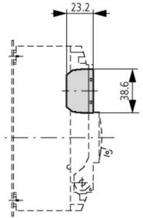
Pushbutton with M22-(C)K... Pushbutton with M22-(C) LED... + M22-XLED...
