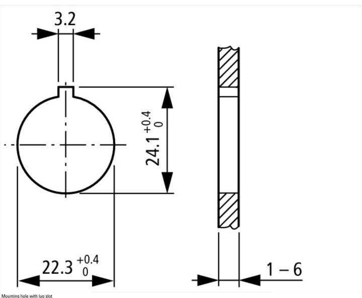
Mounting hole with lug slot
