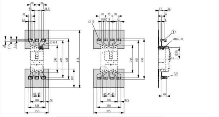
① NZM3(-4)-XK22X21 ② NZM3(-4)-XK300 Length with phase isolators approx. 599 mm
