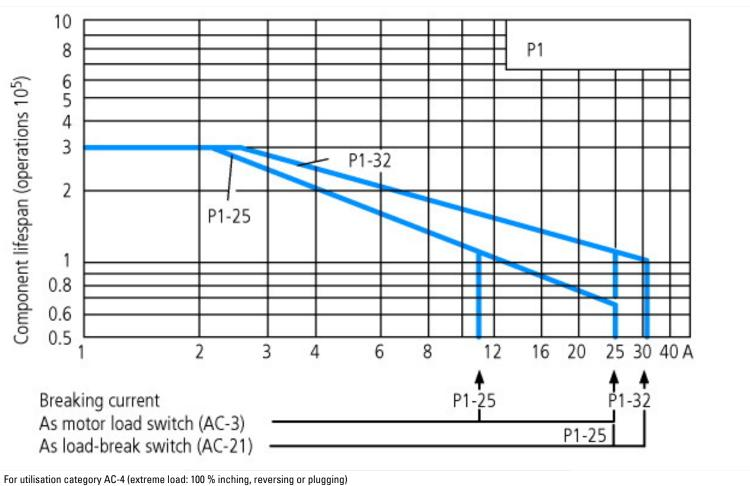
The blocked rotor current of the motor should not exceed the rated current of the switch for AC-21A to ensure a reasonable device lifespan.
