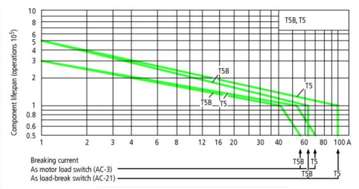
For utilisation category AC-4 (extreme load: 100 % inching, reversing or plugging) The blocked rotor current of the motor should not exceed the rated current of the switch for AC-21A to ensure a reasonable device lifespan.
