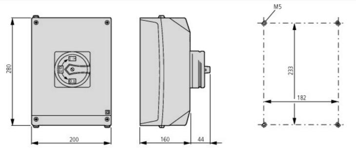
Depth of one contact unit: 16.5 mm The rotary switches T5B and T5 are of identical design but differ in their contacts.
