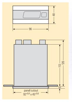
The modular DIGEM 96 x 48 B5 installation measurement instrument is extremely easy to program.
