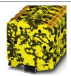
High-current terminal block, Connection method: Power-Turn connection, Cross section: 25 mm² - 95 mm², AWG: 4 - 3/0, Width: 25 mm, Height: 99.8 mm, Color: black/yellow, Mounting type: NS 35/15
