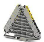
Potential distributors, without actuation lever, nom. voltage: 250 V, nominal current: 17.5 A, cross section: 0.14 mm² - 2.5 mm², AWG: 14 - 26, connection method: Push-in connection, number of positions: 2, number of connections: 32, width: 8.3 mm, length: 100 mm, color: gray, color of connection elements: yellow, black, mounting: NS 35/7,5, NS 35/15
