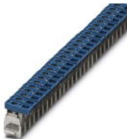
Connection terminal block, Connection method Screw connection, Load current : 76 A, Cross section: 1.5 mm 2 - 16 mm 2 , Width: 9.8 mm, Color: blue
