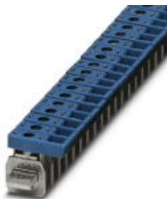
Connection terminal block, Connection method Screw connection, Load current : 41 A, Cross section: 0.5 mm 2 - 6 mm 2 , Width: 7 mm, Color: blue
