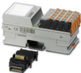
Axioline F analog input module, 8 inputs: 0 - 10 V, ±10 V, 0 - 20 mA, 4 - 20 mA, ±20 mA, 2-wire connection method (including bus base module and connectors)
