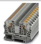
Feed-through terminal block, Connection method: Push-in connection, Cross section: 0.5 mm² - 25 mm², AWG: 20 - 4, Width: 12.2 mm, Color: blue, Mounting type: NS 35/7,5, NS 35/15
