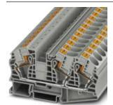
Feed-through terminal block, Connection method: Push-in connection, Cross section: 0.5 mm² - 25 mm², AWG: 20 - 4, Width: 12.2 mm, Color: gray, Mounting type: NS 35/7,5, NS 35/15
