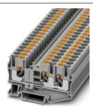
Feed-through terminal block, connection method: Push-in connection, number of connections: 3, cross section:0.5 mm² - 10 mm², AWG: 20 - 8, width: 8.2 mm, height: 42.2 mm, color: gray, mounting type: NS 35/7,5, NS 35/15
