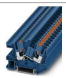
Installation terminal block, Push-in connection, cross section: 0.5 mm² - 10 mm², AWG: 20 - 8, width: 8.2 mm, color: blue, mounting type: NS 35/7,5, NS 35/15
