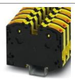
High-current terminal block, nom. voltage: 1000 V, nominal current: 125 A, connection method: Power-Turn connection, number of connections: 2, cross section:2.5 mm² - 35 mm², AWG: 12 - 2, width: 16 mm, color: black/yellow, mounting type: NS 35/15
