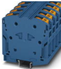
High-current terminal block, Connection method: Power-Turn connection, Cross section: 25 mm 2 - 95 mm 2 , AWG: 4 - 3/0, Width: 25 mm, Color: blue, Mounting type: NS 35/15
