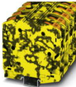
High-current terminal block, Connection method: Power-Turn connection, Cross section: 25 mm 2 - 95 mm 2 , AWG: 4 - 3/0, Width: 25 mm, Height: 99.8 mm, Color: black/yellow, Mounting type: NS 35/15
