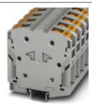
High-current terminal block, Connection method: Power-Turn connection, Cross section: 25 mm² - 95 mm², AWG: 4 - 3/0, Width: 25 mm, Color: gray, Mounting type: NS 35/15
