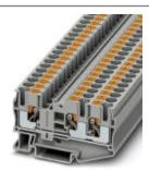
Feed-through terminal block, Connection method: Push-in connection, Cross section: 0.5 mm² - 10 mm², AWG: 20 - 8, Width: 8.2 mm, Height: 42.2 mm, Color: gray, Mounting type: NS 35/7,5, NS 35/15
