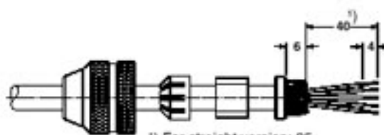
Strip conductor, widen shield and lay around the shielding ring, cut off projecting mesh.
