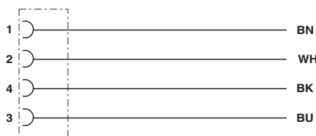
Contact assignment of the M12 socket
