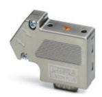
D-SUB plug, 9-pos. socket, two cable entries less than 35° to two terminal block rows, bus system: CAN, CANopen, SafetyBUS p up to 1 Mbps, termination resistor can be switched on via slide switch, pin assignment: 2,3,7,9; screw connection terminal blocks
