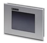
Touch panel with 16.5 cm (6.5") graphics-capable TFT display, 65,535 colors, 640 x 480 pixels, 1 x Ethernet, 2 x USB, and integrated runtime of the Visu+ visualization software.
