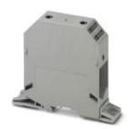
High-current terminal block, nom. voltage: 1000 V, nominal current: 309 A, connection method: Screw connection, number of connections: 2, cross section: 35 mm² - 150 mm², AWG: 2 - 300 kcmil, width: 31 mm, height: 111 mm, color: gray, mounting type: direct screw connection
