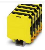
High-current terminal block, nom. voltage: 1000 V, nominal current: 150 A, connection method: Screw connection, number of connections: 2, cross section: 16 mm<sup>2</sup> - 70 mm<sup>2</sup>, AWG: 6 - 2/0, width: 20 mm, color: black/yellow, mounting type: NS 35/7,5, NS 35/15, NS 32, NS 35/15-2,3
