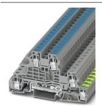
Installation ground terminal block, nom. voltage: 400 V, nominal current: 38 A, Screw connection, Rated cross section: 6 mm², cross section: 0.2 mm² - 10 mm², mounting type: NS 35/7,5, NS 35/15, color: gray
