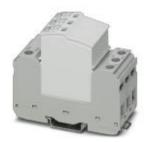
Plug-in surge arrester, in accordance with Type 2/Class II, for 3-phase power supply networks with combined PE and N installed in one conductor (4-conductor system: L1, L2, L3, PEN), with remote indication contact.
