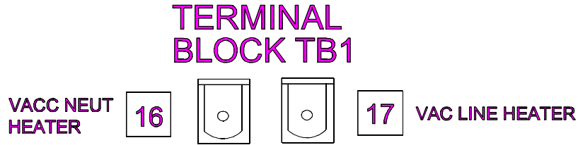
Figure 3a. Heater option connection for 19" Rack Mount unit
